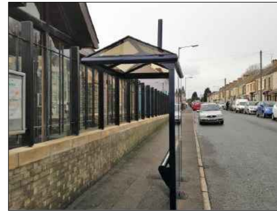
Example of 2 bay cantilever bus shelter to be located in Church Lane (to be located at back of path facing out, perch seat)
